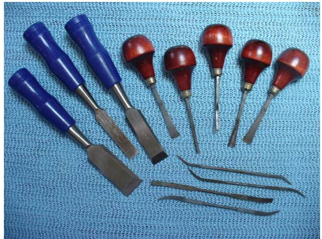
Photo 1: Woodcarving tools including chisels and gouges.
