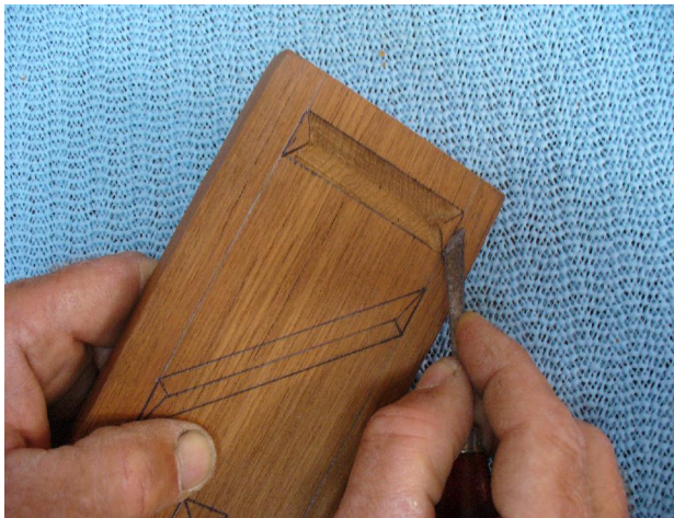
Photo 10 : The same 45-degree angle should be maintained. Then gently...very gently... slice along the top vertical line.
