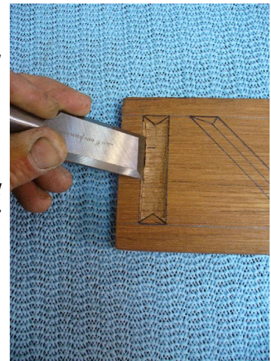
Photos 7 & 8: Lightly tap the chisel with the mallet two or three times and move the chisel to the next part of the line and repeat. Rotate the board and repeat until you have formed a v-shaped trough with a clean line at the bottom.
