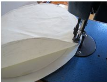
Sewing the plastic disc between two pieces of sail canvas.
