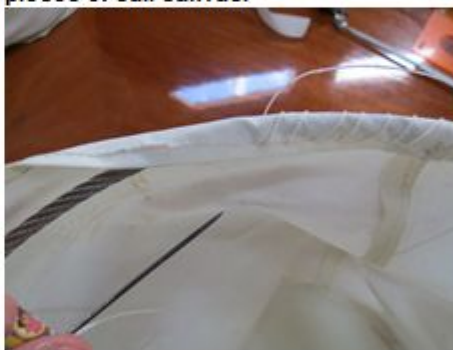
Sewing the plastic disc between two pieces of sail canvas.
